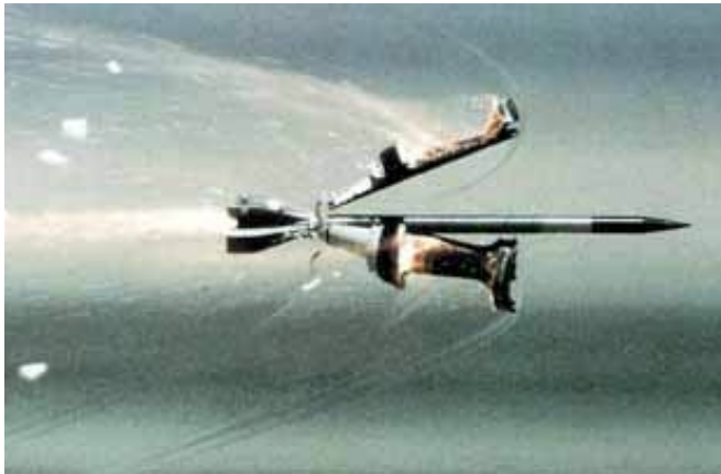
Figure 1: Armor-piercing ammunition shortly after being fired, at the moment of release from its sabot.
